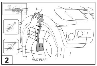
Remove the mud flaps by removing and retaining the 7 scrivets from inside the wheel arch as shown.
