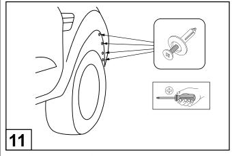
Remove all 4 scrivets from the wheel arch on front bumper.
