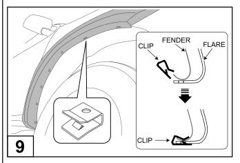
Install the wide clip at an angle, by pushing it on to the fender lip and then rotate downwards, as shown.
