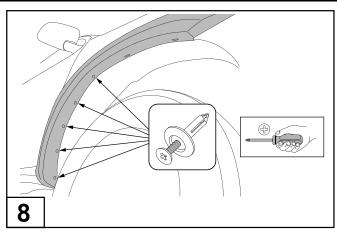
Install 5 wheel arch scrivets onto the flare as shown. While pressing and holding the flare in position of best fit.
