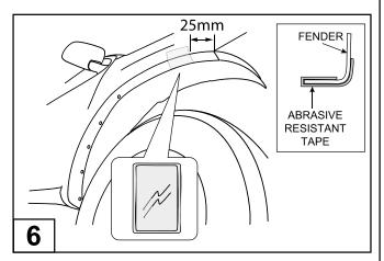
Cut in half the anti-abrasive tape and apply to the front fender as marked 25mm from the front bumper bar. Ensure you wrap the abrasive tape strip down around the lower edge of the fender onto the inside.
