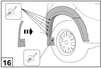
Secure the mud flap to the fender flare with 5 scrivets and 1 to the plastic splash guard, as shown.
