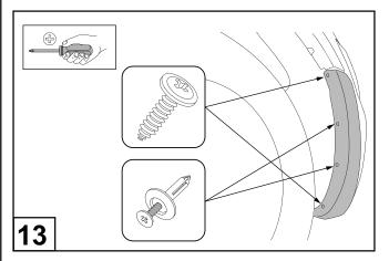
Secure the fender flare to the bumper with 2 Phillips head screws and 2 scrivets as shown.
