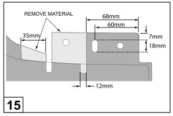
Measure and mark slot position and mud flap area to be removed, as shown. Using tin snips remove the light grey area. Cut 6x18mm slot using die grinder.
