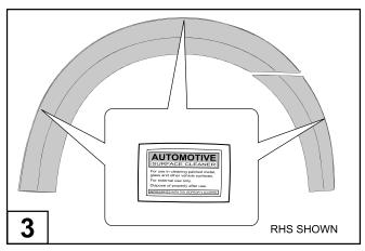
Clean the inside edge of each fender flare where the rubber extrusion will adhere.
