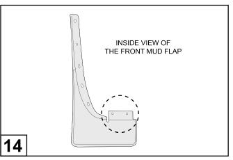
Prepare the mud flap by cleaning it and covering marked area with a masking tape.
