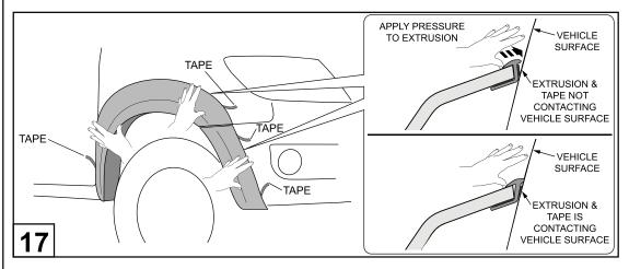
Ensure that flares are aligned. Remove the tape liner. Using your thumb and/or fingers apply firm pressure on the extrusion to ensure the extrusion and the tape is contacting the vehicle surface around the full perimeter of the flares.
