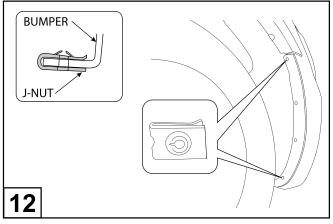
Hold the splash guard inwards and push the supplied 2 J-nuts onto the front bumper in the top and bottom hole position as shown.
