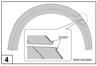
Remove approximately 50mm of the protective liner from the extrusion. Fit the extrusion to the Fender Flare along the edge that comes in contact with the vehicle's body panel. NOTE: Start applying the extrusion from area show above.
